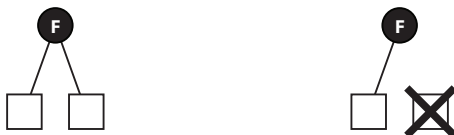
Fig. 2. Generic representation of redundancy. Left: The function F can be realised by two (or possibly more) components which either share the load synchronously (as shown here), or realise the function independently and asynchronously (with one being used whilst the other is spare). Right: When one of the components fails (as indicated by the X), the function is realised by the other component (as shown here), or the function 'switches' from one of the components to the other.
