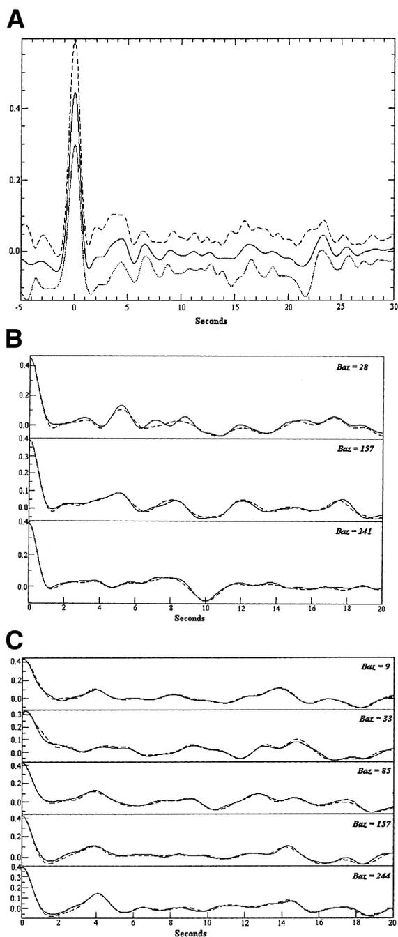
Fig. 4. (A) The solid line represents the stack of all the observed receiver functions and the broken lines are the limits for all receiver functions at LSZ. (B) Observed (broken line) and synthetic (solid line) receiver functions for LBTB. (C) Observed (broken line) and synthetic (solid line) receiver functions for BOSA.
