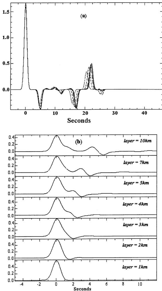
Fig. 7. Plots of receiver functions from a forward modelling procedure to investigate the minimum shear wave velocity that can receiver produce a change on the function (a) and the minimum resolvable layer thickness (b).
