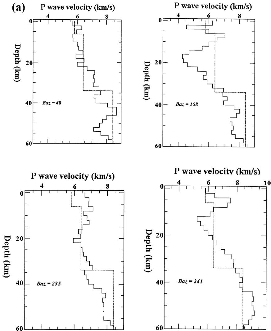
Fig. 5. (A) Inversion results for LSZ. (i) Solid line is the average velocity model and the broken lines represent the standard deviation, (ii) observed (solid line) and synthetic (broken lines) receiver functions from the four starting models. (B) Inversion results for LBTB and BOSA. The solid line model is the average of models from northeast, southeast and southwest quadrants. The broken line models are the standard deviation.
