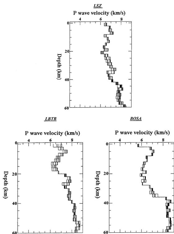
Fig. 6. Twelve acceptable velocity models resulting from 120 waveform inversions of the southwest radial receiver function at each of the stations, LSZ, LBTB and BOSA. Each model produces a synthetic waveform that compares well to the observed receiver functions
