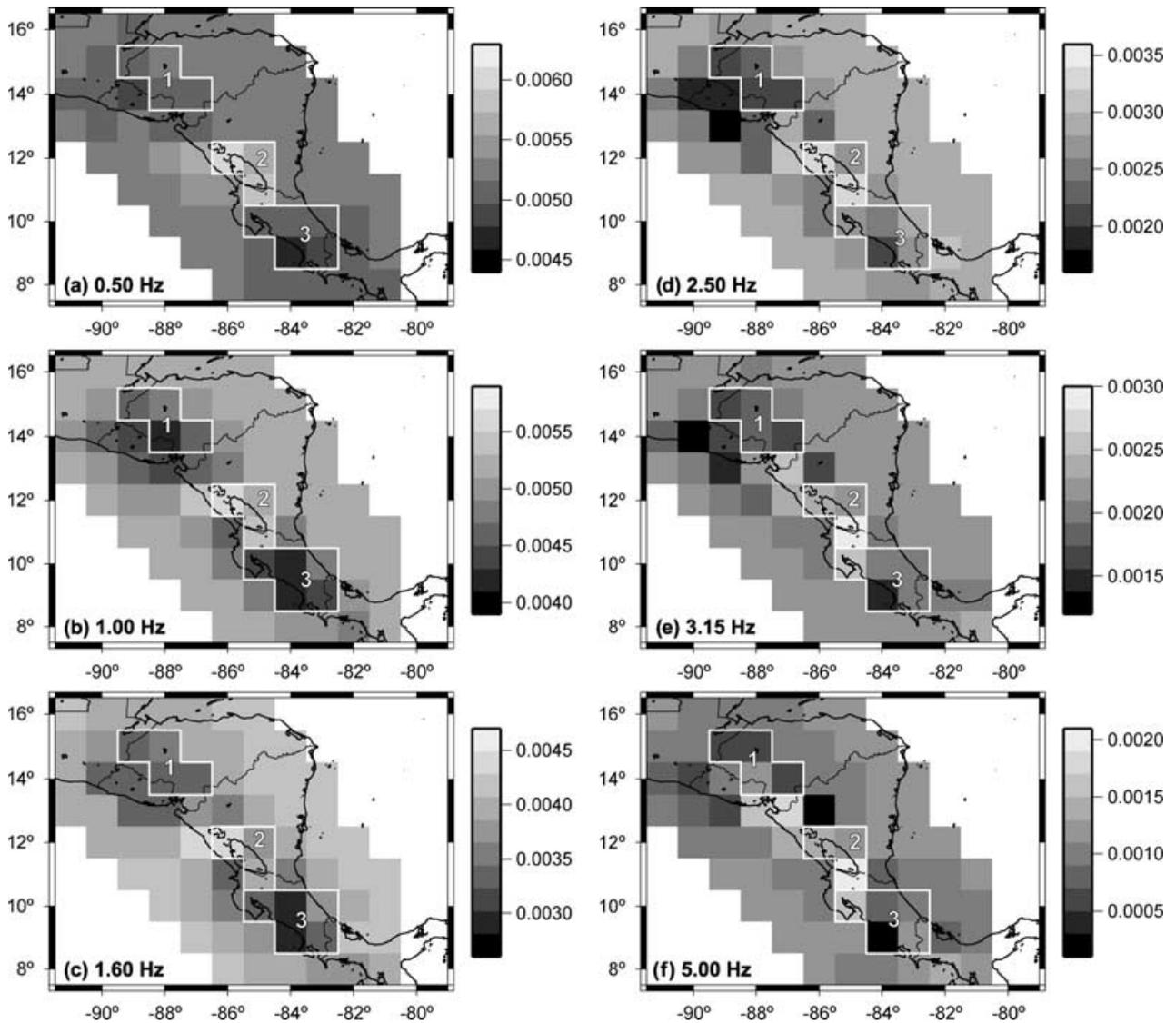
**Figure 5.** Result of the tomographic inversion for  $Q_{Lg}^{-1}$  in Central America at (a) 0.5 Hz, (b) 1.0 Hz and (c) 1.6 Hz. The travel paths used are shown in Fig. 1. The lines and numbers show the grouping of grid cells into regions of similar  $Q_{Lg}^{-1}$  values: (1) western Honduras, (2) Nicaraguan Depression and (3) Costa Rica. Result of the tomographic inversion for  $Q_{Lg}^{-1}$  in Central America at (d) 2.5 Hz, (e) 3.15 Hz and (f) 5.0 Hz.
