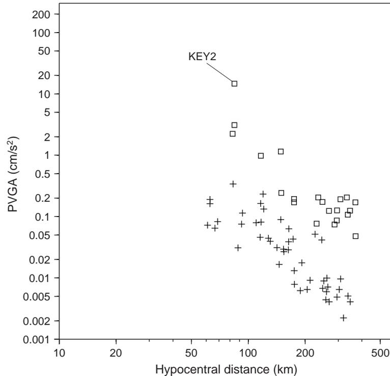
Fig. 13. The decay of vertical ground acceleration (PVGA) with hypocentral distance for the mainshock (squares) and the largest aftershock (crosses).
