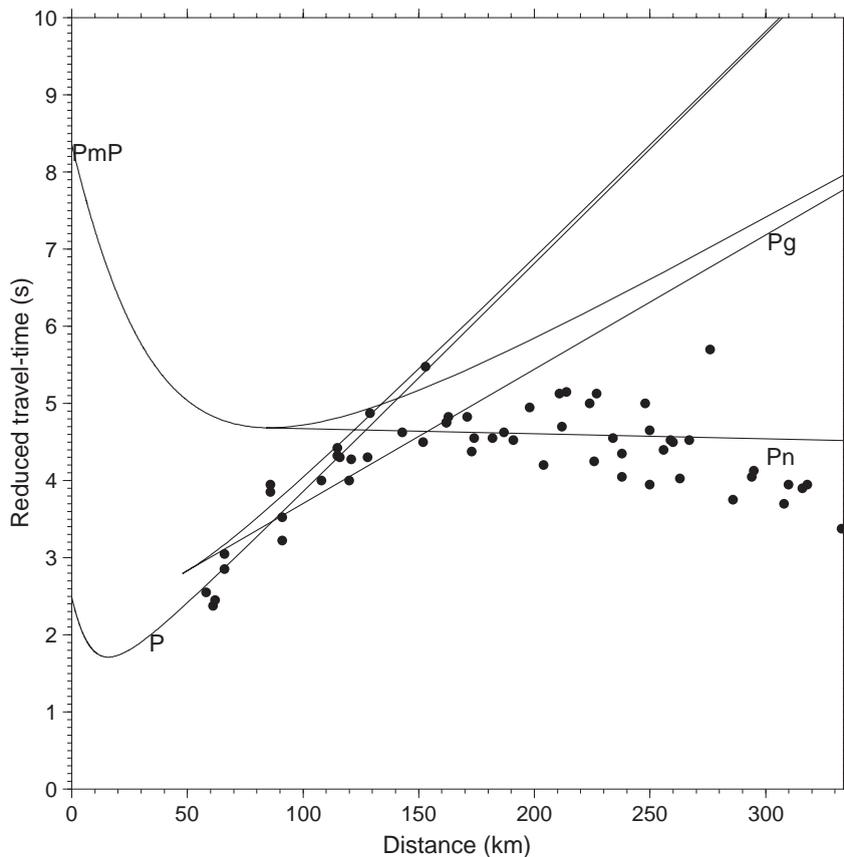
Fig. 4. Reduced  $P$ -wave travel times for the Dudley earthquake as a function of epicentral distance for both observed (black circles) and modelled data. Theoretical  $P$ -wave travel-time curves for primary crustal phases are determined for the 1-D velocity model used to locate the earthquake and a source depth of 14 km. The data have been reduced using a reduction velocity of 8 km/s.
