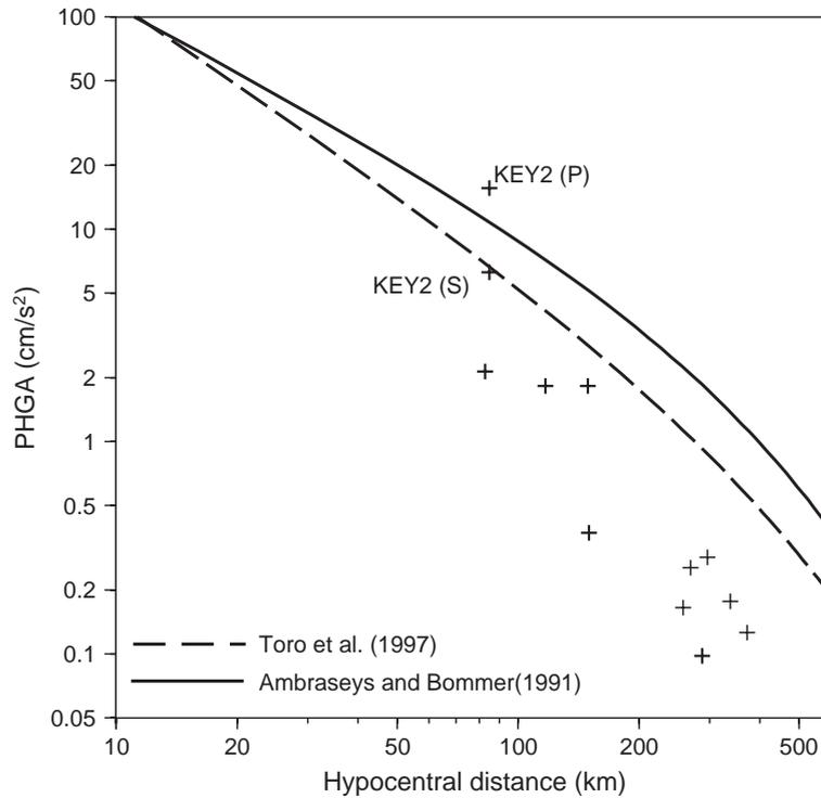
Fig. 14. Observed values of peak horizontal ground acceleration (PHGA) for the mainshock from strong motion (triangles), short period (circles) and broadband instruments (squares), compared with the values predicted by (Ambraseys and Bommer, 1991) (solid line) and (Toro et al., 1997) (dashed line).
