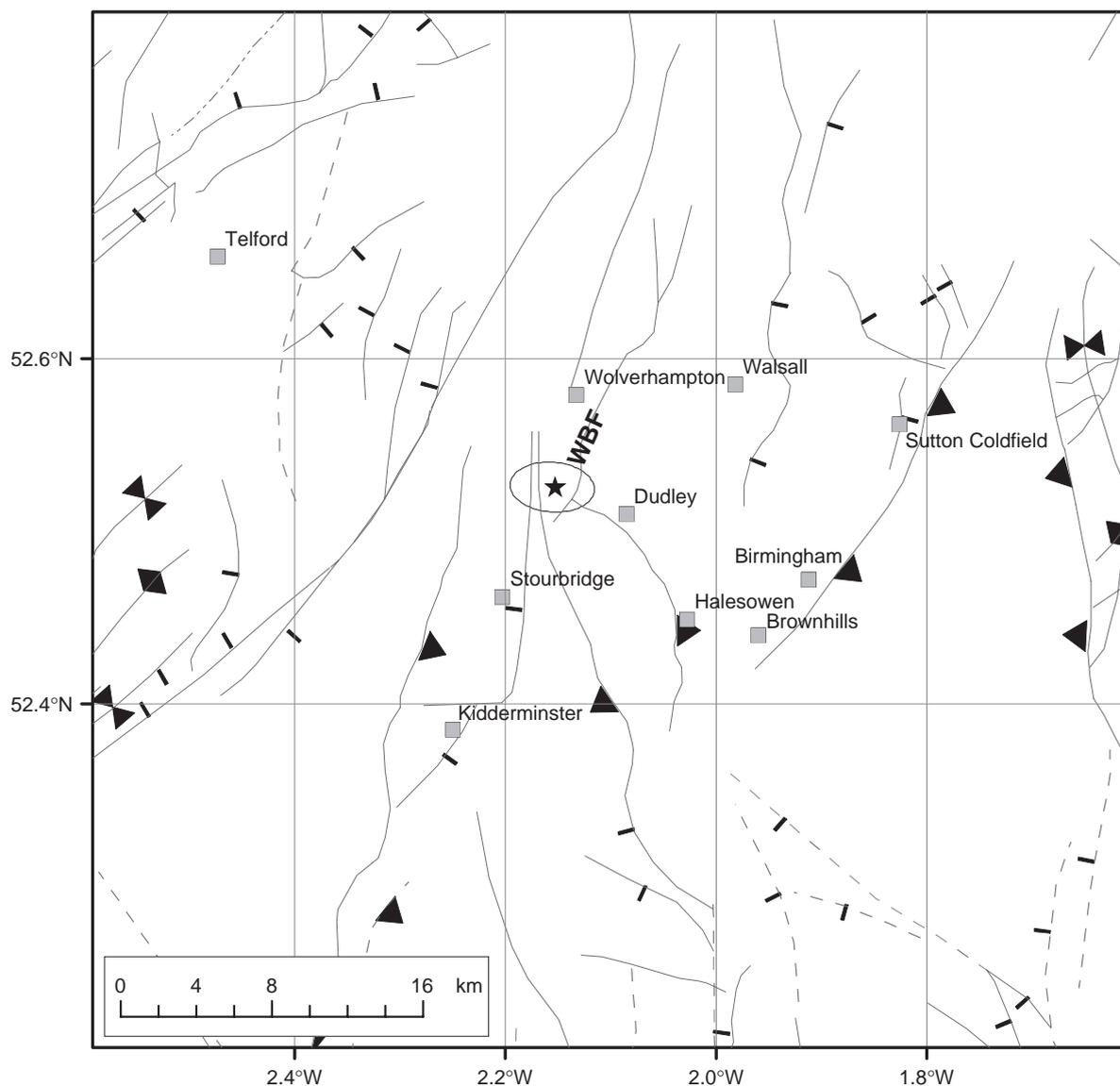
Fig. 3. Horizontal projection of the 90% confidence ellipsoid for the calculated hypocentre of the Dudley earthquake (marked by the star), along with surface trends of the principal faults in the West Midlands. Normal faults are denoted by a square on the downthrown side, while reverse faults are denoted by a barb on the upthrown side. The Western Boundary Fault is denoted by WBF.
