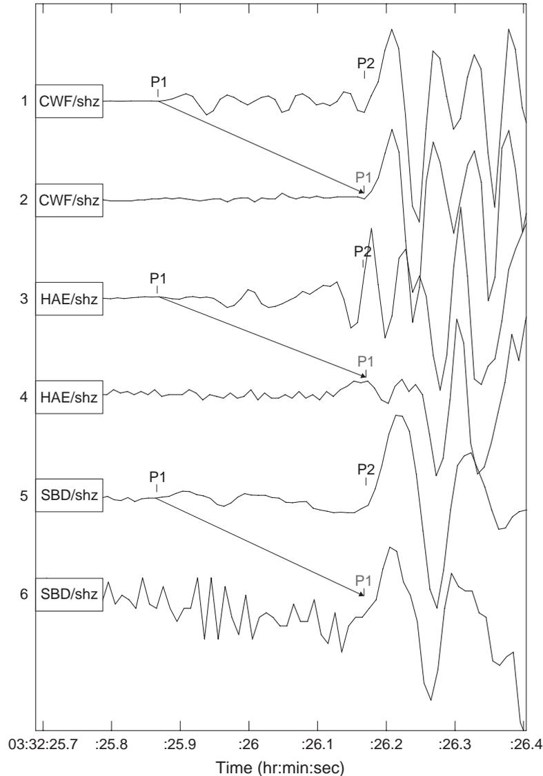
Fig. 10. Ground velocity seismograms from the first aftershock at 03:32 UTC on 23 September. The precursory signal has been aligned in time and scaled by a factor of 10 to the same amplitude as the larger arrival to show the similarity of the signals at the three stations CWF, HAE and SBD.
