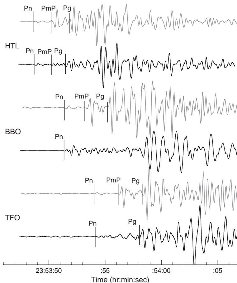
Fig. 9. Observed (black) and modelled (grey) ground displacement seismograms for stations AEU (230 km), HTL (234 km), BBO (256 km) and TFO (276 km). The synthetics were generated using a source depth of 14 km.
