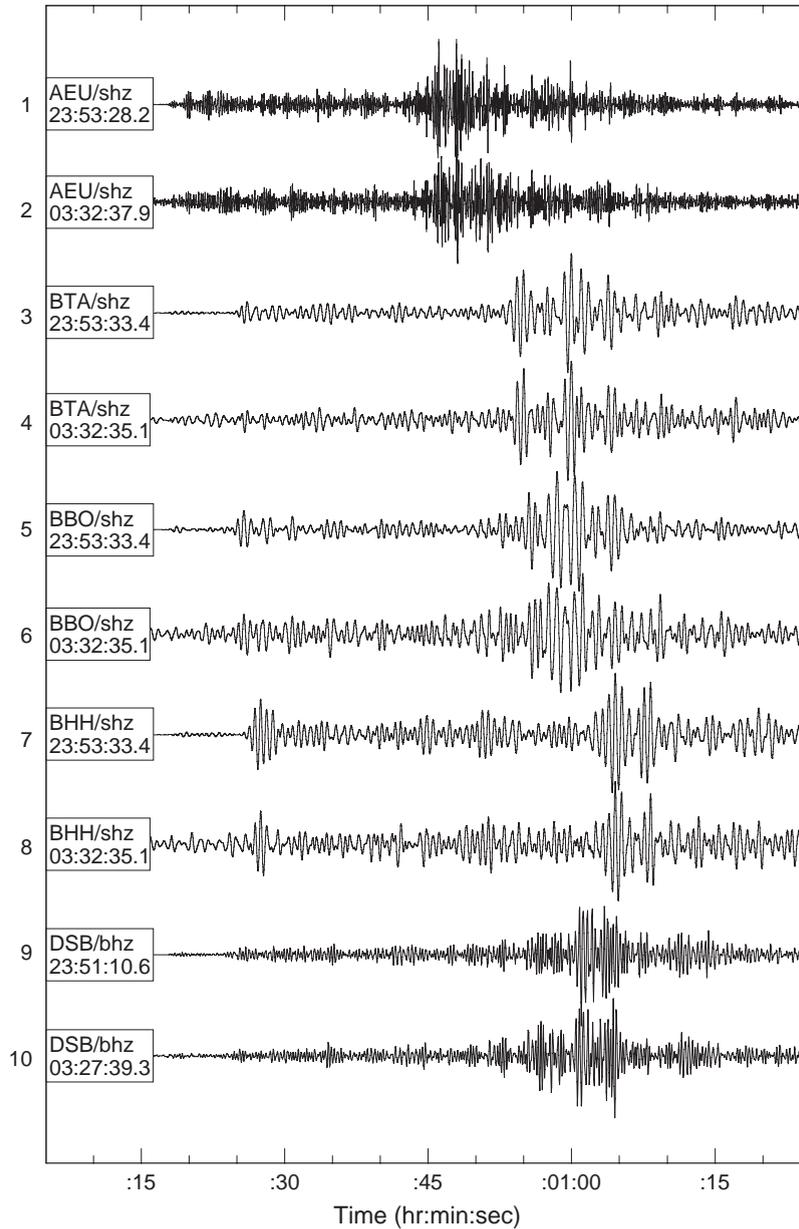
Fig. 11. A comparison of the waveforms from the mainshock and the first aftershock at 03:32 UTC on 23 September. All traces have been band-pass filtered: trace numbers 1, 2, 9 and 10 are filtered from 3 to 8 Hz; trace numbers 3 to 8 are filtered from 2 to 4 Hz.
