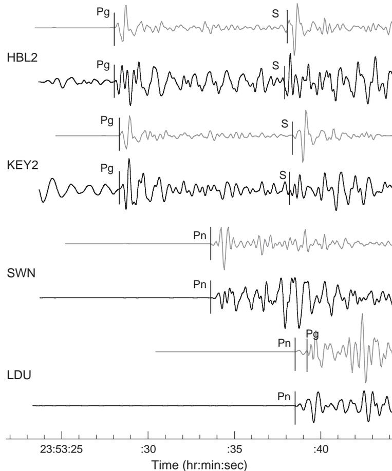
Fig. 8. Observed (black) and modelled (grey) ground displacement seismograms for stations HBL2 (80 km), KEY2 (82 km), SWN (115 km), LDU (148 km) and WOL (149 km). The synthetics were generated using a source depth of 14 km.
