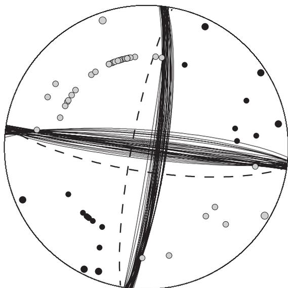
Fig. 6. Source mechanisms determined for the Dudley earthquake using first motion polarities from local recordings. The best-fitting double-couple solution given by moment tensor inversion of regional broadband waveforms obtained by the Swiss Seismological Service is shown by the dashed lines.
