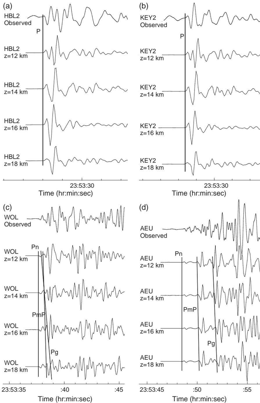
Fig. 7. Observed and modelled ground displacement seismograms for four source depths of 12, 14, 16 and 18 km at stations (a) HBL2, epicentral distance 80 km, (b) KEY2, epicentral distance 82 km, (c) WOL, epicentral distance 149 km, (d) AEU, epicentral distance 230 km. A band-pass filter of 1–4 Hz has been applied to the data.
