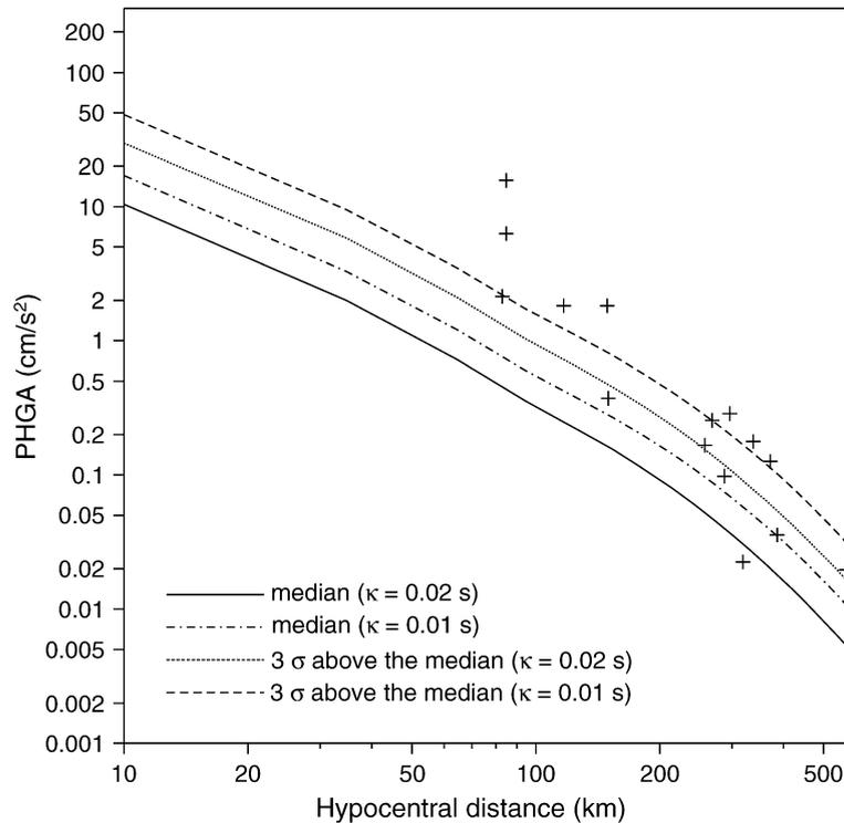
Fig. 15. Comparison of observed PHGA for the mainshock with theoretical values using RVT. Crosses show the observed data. The solid black line shows PHGA calculated using average  $\Delta\sigma$  and  $M_w$  from Table 3 and  $\kappa=0.02$ . The dotted line shows a more conservative estimate of PHGA calculated using the standard deviation on  $\Delta\sigma$  and  $M_w$ .
