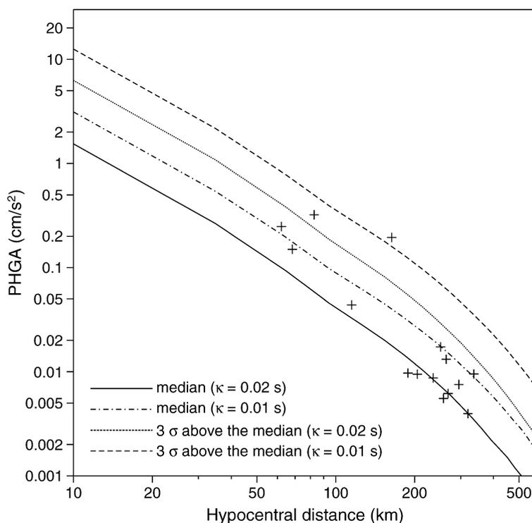
Fig. 16. Comparison of observed and theoretical PHGA for the first aftershock. Crosses show the observed data. The solid black line shows PHGA calculated using average  $\Delta\sigma$  and  $M_w$  from Table 4. The dotted line shows a more conservative estimate of PHGA calculated using the standard deviation on  $\Delta\sigma$  and  $M_w$ .
