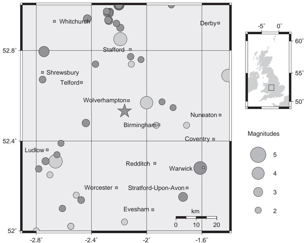
Fig. 1. Instrumental (dark circles) and historical (light circles) seismicity of the West Midlands from 1768 to the present, in a 100 km<sup>2</sup> centred on the 2002 epicentre, marked by the star.
