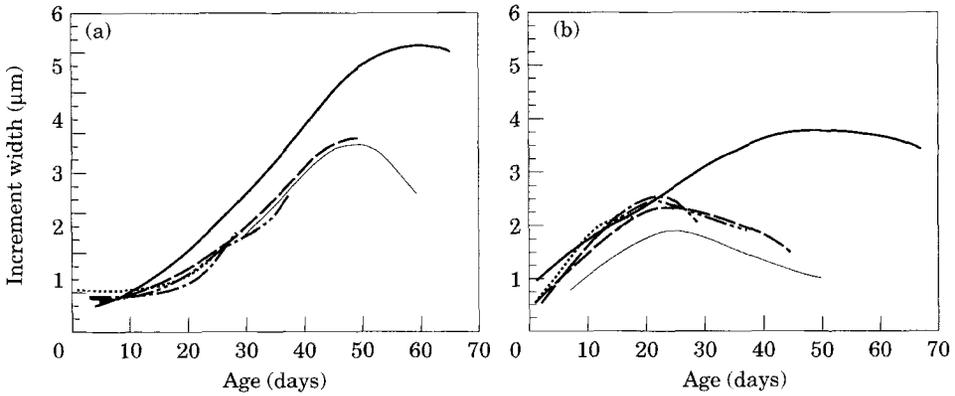
FIG. 4. Age-specific otolith growth of herring larvae in (a) mesocosm A and (b) mesocosm B (increment widths in  $\mu\text{m}$ ). Lines are estimated by distance weighted least squares fit. Larvae are grouped into categories based on age of capture (days after hatching):  $\cdots$ , 10–19;  $-\cdot-\cdot-$ , 20–29;  $-\cdot-\cdot-$ , 30–39;  $-\cdot-\cdot-$ , 40–49;  $-\cdot-\cdot-$ , 50–59;  $-\cdot-\cdot-$ , 65–67.
