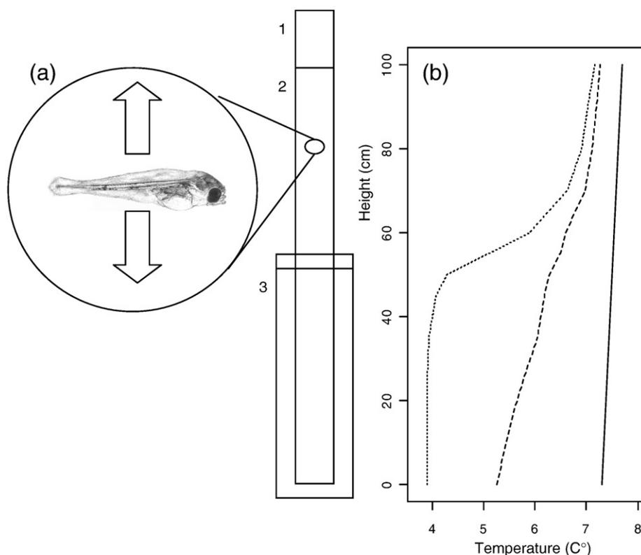
**Fig. 1.** (a) Simplified illustration of experimental design showing the plastic bag (1), the water level (2) and the level of the thermocline (3), (b) the plot of the characteristics of the thermoclines scaled to the illustration. Illustration of cod larvae by Laura Vollset.
