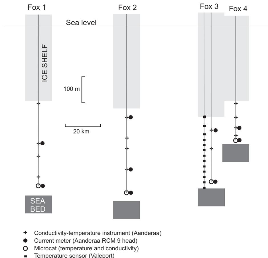
**Figure 2.** Diagram showing moorings deployed during 2002-03. Thermistor cables deployed at Fox 3 and Fox 4 are not shown.
