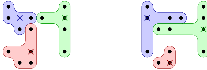
Fig. 1. Optimal clusterings of the same set of vectors with different distances: \text{dist}_1 in the left subfigure, \text{dist}_{1/4} in the right subfigure. Shapes denote clusters, crosses denote cluster centroids.
