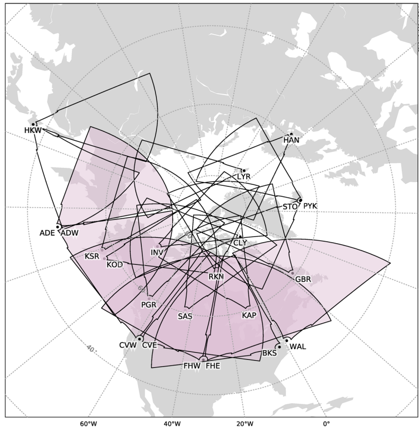
Figure 1. Fields of view of the Northern Hemisphere Super Dual Auroral Radar Network radars highlighting the eight North American midlatitude radars used in this study.
